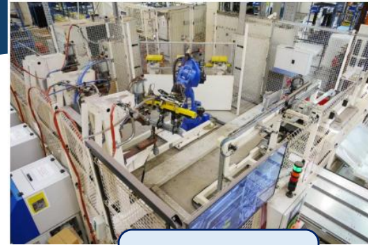
Resistance welding line
